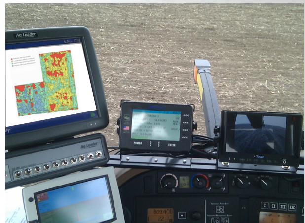
Tractor guidance system using the shapefile map
